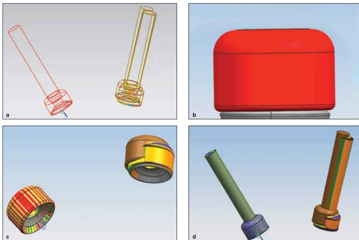
**Fig 3** The individual virtual mating cylinders representing the scanned positions of implants. (a) The scanned implant positions. (b) A virtual single-screw lift test was created in the second mating cylinder. (c) Distance measurements were taken from the center point of virtual mating cylinders. (d) Angular measurements were taken from the vertical axes of mating cylinders.
