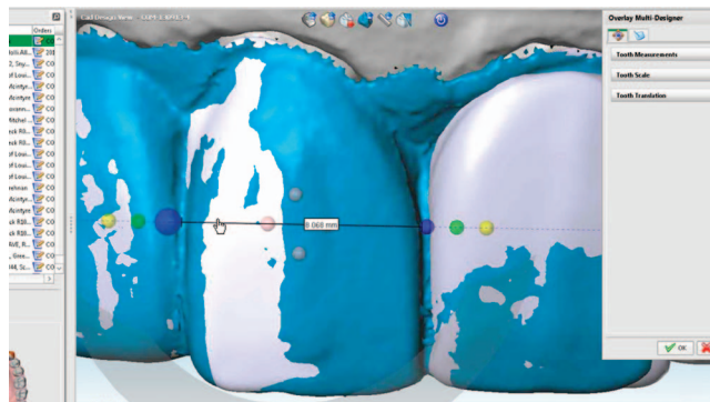
Figure 11. The digital ruler was used to ensure the dimensions of the designs for the future CAD/CAM-fabricated lithium disilicate ceramic veneers. The three-dimensional measurements on the CAD should have a close resemblance to the virtual esthetic plan-guided diagnostic wax-up.
